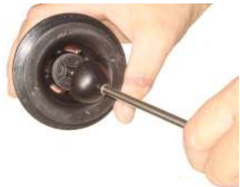
Pull gently on the shaft to separate the dome connector from the aeration pump.
