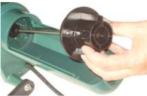
Gently lift the black plastic aeration pump and pull the shaft away from the motor coupling.
